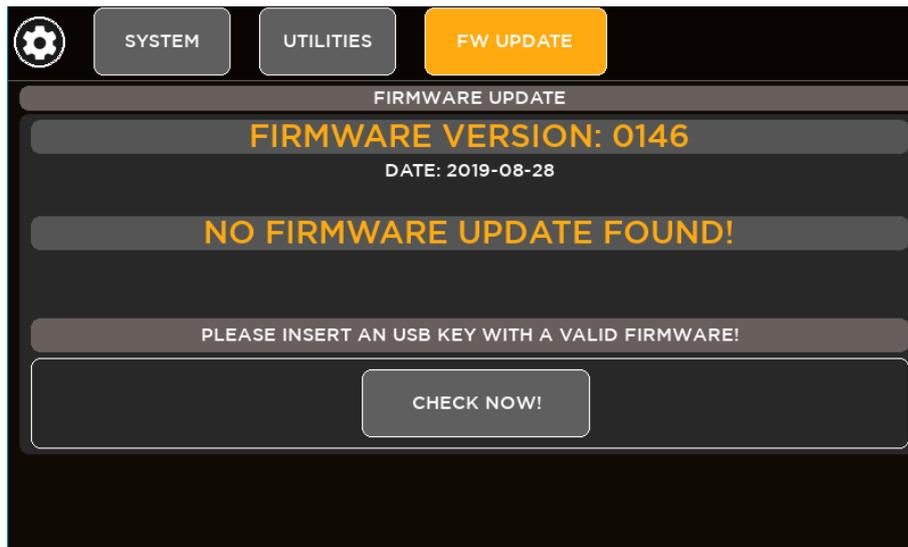
5. Insert your USB stick into the USB A port. The upper side shows the firmware version that is currently installed on the mixer. The bottom side shows the firmware version on the USB stick ready to be installed.
