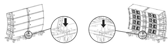
It is recommended to clasp the karts with the appropriate hook (as shown in the picture), for a stable and safe transportation.
