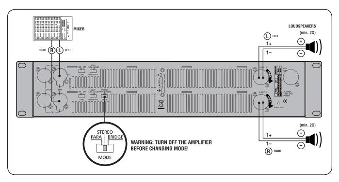
As alternative wiring, the amplifier output 2 is also available on the SPEAKON connector of the output 1 (pins: 2+ positive, 2- negative).
