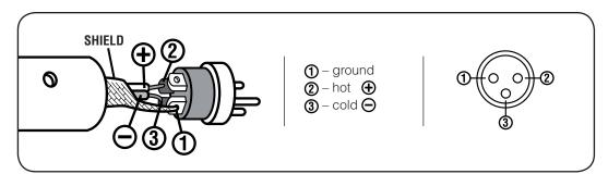
8 Balanced parallel audio output (one per channel, male XLR connector)
