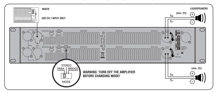
As alternative wiring, the amplifier output 2 is also available on the SPEAKON connector of the output 1 (pins: 2+ positive, 2- negative).
