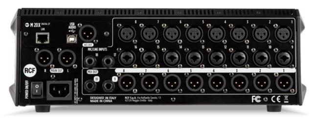
On the M 20X rear panel, 8 Mic inputs equipped with XLR connector and 8 Mic/Line inputs with COMBO connectors are available, with two additional TRS jacks line inputs. The MIX output section includes 8 male XLR and 2 TRS jacks on which all the internal audio output paths can be routed. A pair of male XLR, preassigned to the Main Mix output, and an assignable
