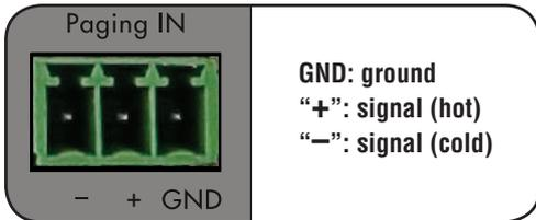
**1a** “Paging IN”: balanced audio input (with “Phantom” power supply when both “Phantom” DIP switches are set to ON) for either a paging microphone (when both “Line/Mic” DIP switches are set to “Mic”) or a “line” signal for announcements (when both “Line/Mic” DIP switches are set to “Line”).
