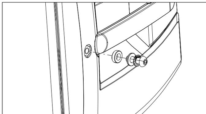
Fix spacers, washers and screws on the upper and lower inserts. Do not completely tighten the screws.
