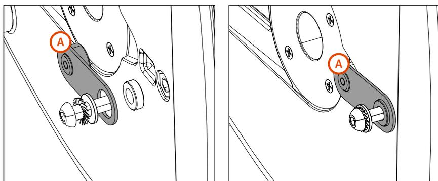
On the lower insert also place the **A** bracket.
