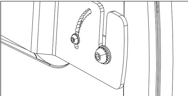
Tighten completely the M10 and M6 screws.
