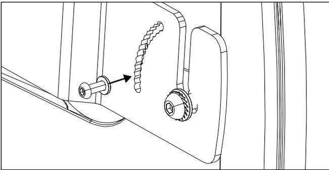
Set the inclination angle with the M6 screw equipped.
